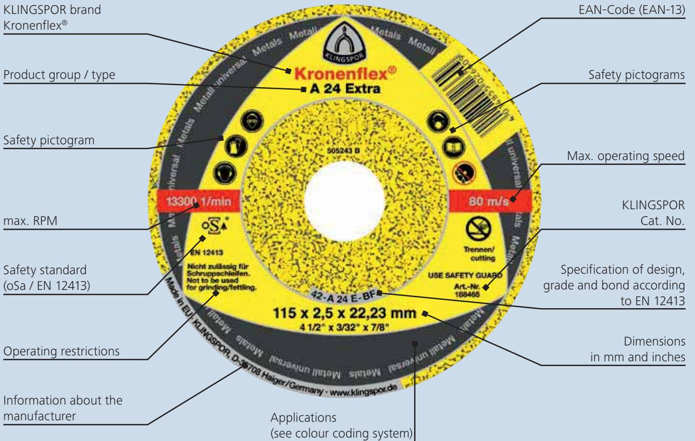
**KLINGSPOR cutting-off wheel and grinding disc colour coding system**
