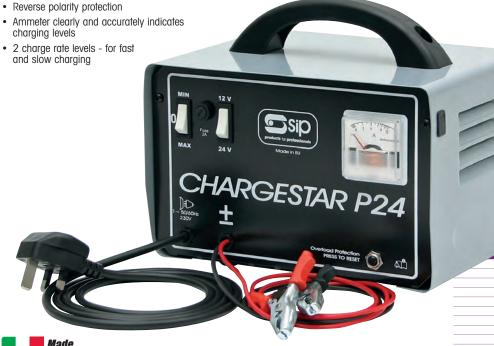
Supply 230v (13amp) 12v / 24v Charging Voltage/s 85Ah 85amps Max. Rated Battery Capacity Rated Output Max. Rated Output Charge Rate Settings Degree of Protection Insulation Class IP20 Weight 5.38kg Packaged Dimensions (HxWxL) 215 x 265 x 300mm
