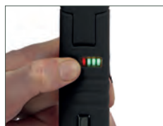
battery test button
