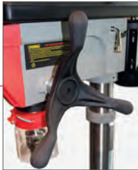
One piece cast 'soft grip' handles
