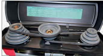
Quick and simple 'easy-lock' motor speed adjustment
