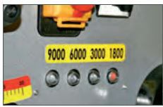
Light display for easy-to-read speed indicator
