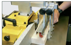
Independently micro adjustable outfeed fence
