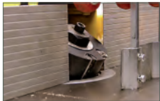
Spindle tilt from -10° to +30°
