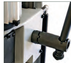
Rise and fall handle features a ratchet mechanism to give optimum leverage
