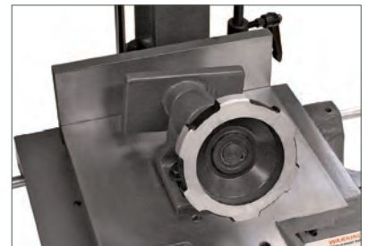
The repositionable cast iron clamp provides a solid hold for a wide range of workpiece sizes
