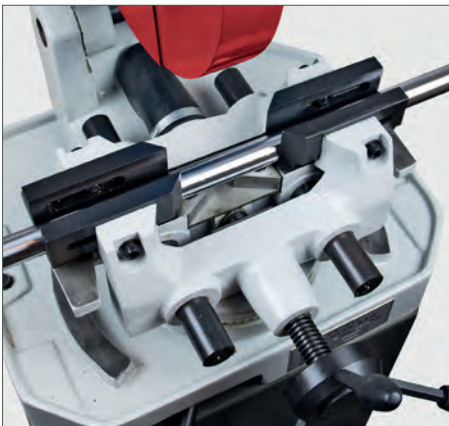
Twin vice - centralises the workpiece
