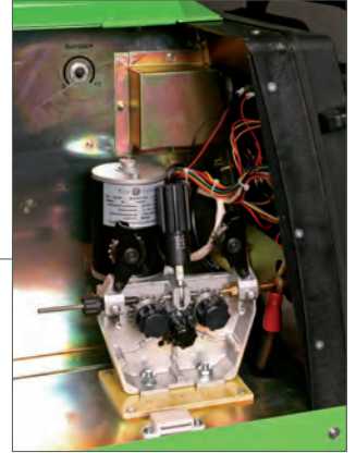
Heavy duty all metal 4 roller wire feed
