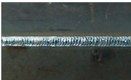
CO2 MIG, flat welding, carbon steel, 130amps
