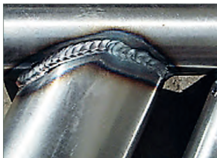
TIG, flat welding, carbon steel, 130amps
