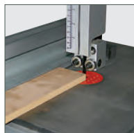
Auxiliary Fence for cutting thinner materials
