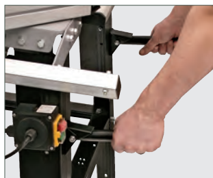
Integrated lifting handles
