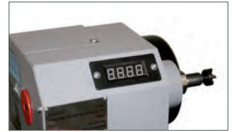
Digital speed read-out display
