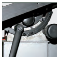
Rack and pinion 45° table tilt
