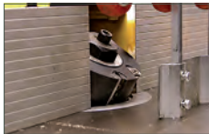
Spindle tilt from -10° to +30°
