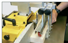
Independently micro adjustable outfeed fence
