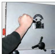
Quick release blade tension
