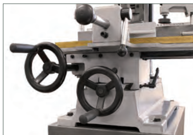
Multi-height, depth table adjustment
