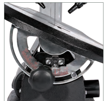
Cast iron table, tilts 0° to 45° left and right
